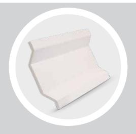
For best results, install one TrueVent unit between roof rafters that are 16" apart. If rafters are 24" apart, use two TrueVent units for maximum ventilation.
